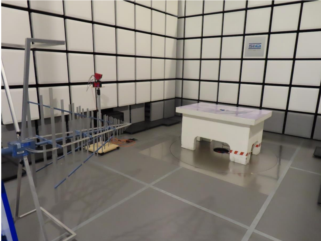
Figure 2: Test setup for radiated emission measurement – up to 1 GHz
