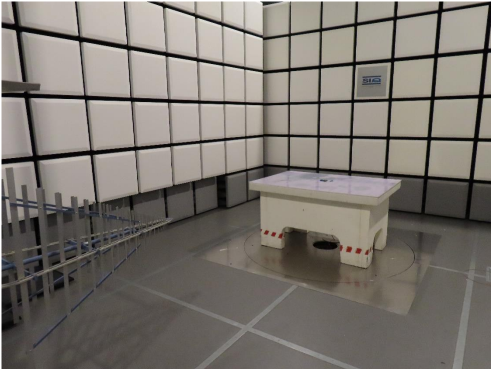
Figure 2: Radiated emission measurement – up to 1 GHz (sample picture for all models)
